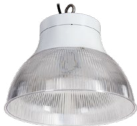
Figure 3: High-output LED modules with a wide-beam optic significantly reduced the number of luminaires required in the refurbishment at Darlington College. This die-cast aluminium body LED module with prismatic polycarbonate diffuser delivers CCT of 4000K and up to 130lmW -1
