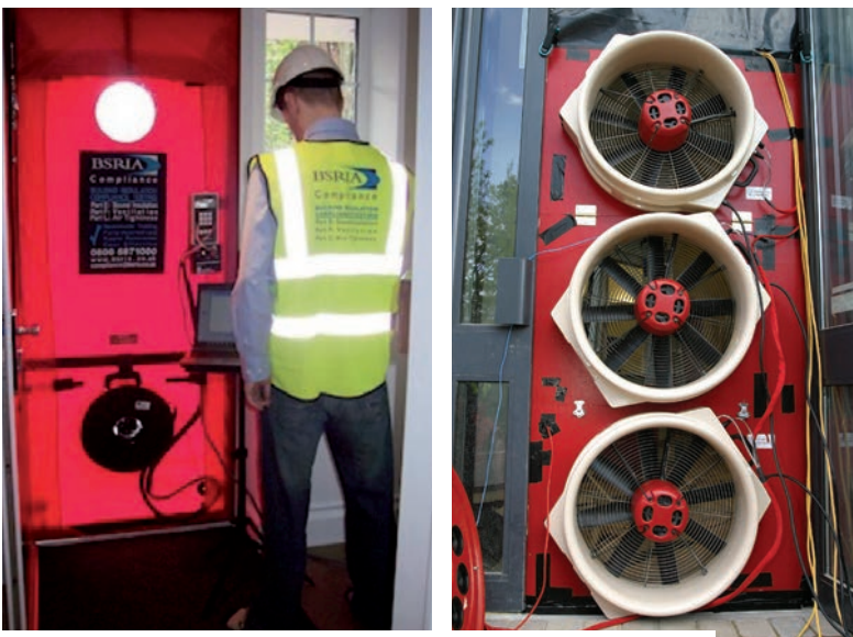
Figure 1: (left) Fan pressurisation equipment typically used in individual dwellings and small buildings for blower door tests, and (right) a multi-fan installation that can be used for large buildings (courtesy of BSRIA)
