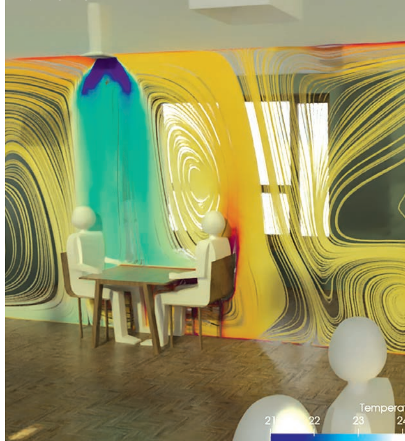
CFD model from SimScale showing cold air entering a room from ceiling diffusers and spreading through the room
