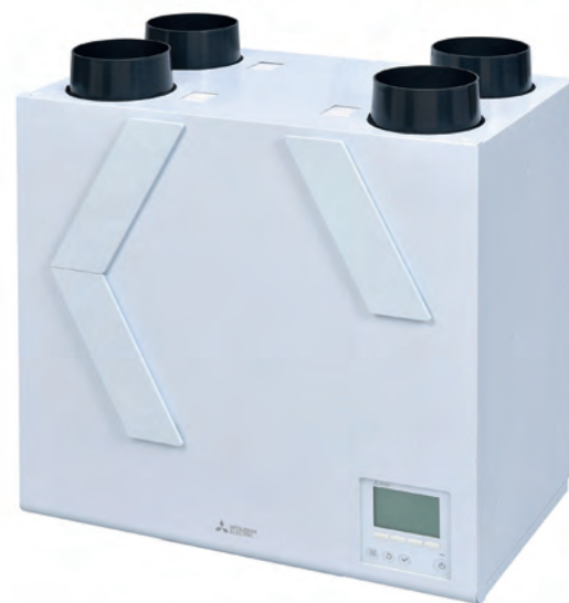
Figure 2: Example of a residential MVHR unit with cross-flow total heat exchanger with efficiency up to 90%, a controllable bypass to prevent unwanted heat exchange, coarse 55% (G3) filters, optional NOx 90% and ePM2.5 50% filtration filters, capable of supplying up to 69L·s -1 (Source: Mitsubishi Electric)
