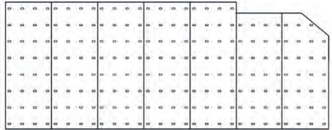
Figure 1: The optimisation process has reduced the amount of roof glazing area from a baseline of 15% to just 4.1%, while still meeting acceptable daylighting requirements' and reducing annual sunlight exposure (ASE) levels to acceptable limits determined by Leed and Well standards
