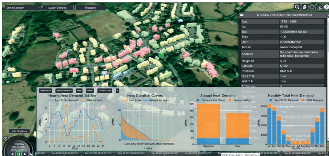
Figure 1: Screenshot of Barcombe's digital twin, with predicted heat demand. The coloured blocks represent different building typologies
