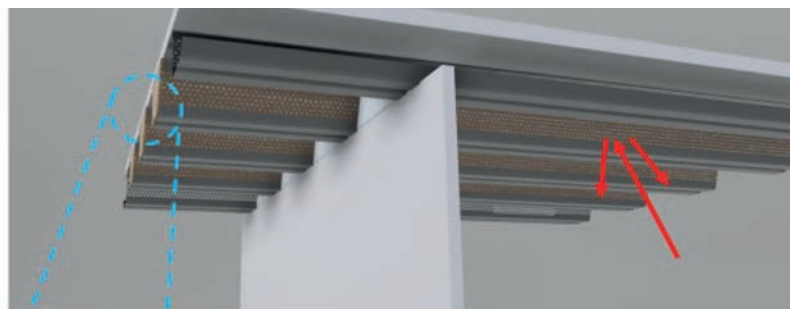
Trapezoidal trays across ceilings fitted with smoke plugs
