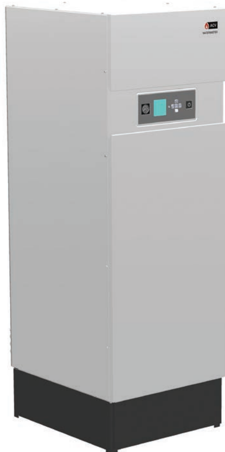
Figure 1: Example of a part-storage gas water heater. This example can provide 440 litres of hot water (with a 50K temperature rise) in the initial 10 minutes and then sustain a continuous flowrate of 29 litres per minute (Source: ACV)
