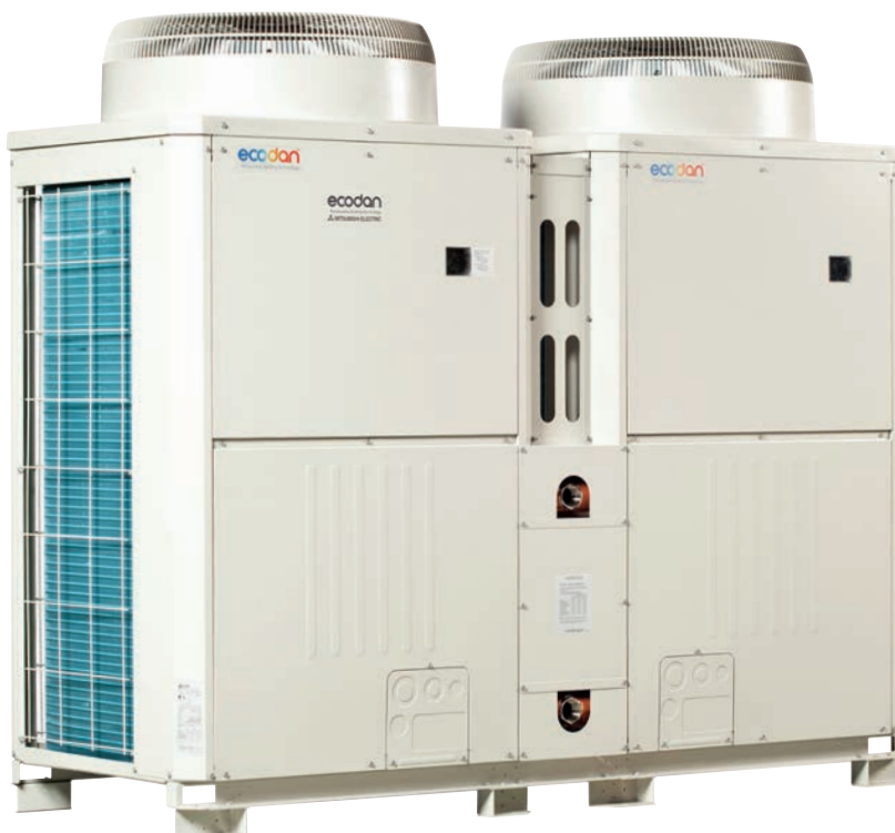
Figure 1: An example of a modular air source heat pump installation that can be used as part of modular systems able to supply from 18kW to 688kW, in 0.5kW increments, with water flow temperatures available from 25°C to 70°C (Source: http://les.mitsubishielectric.co.uk/ )
